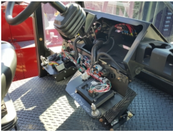
Flip-down Dash with Color/Number Coded Wiring (Standard)
