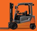
Battery Voltage (V) 80 Load Capacity (lbs.) 4000-7000 Load Center (in.) 24 Maximum lift height (in.) 257.0 Travel speed with/without load (mph)\* 11.8/12.4 Lift speed with/without load (fpm)\* 90.6/124
