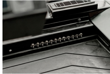
Heavy Duty Circuit Breakers/Reset Switches (Standard)
