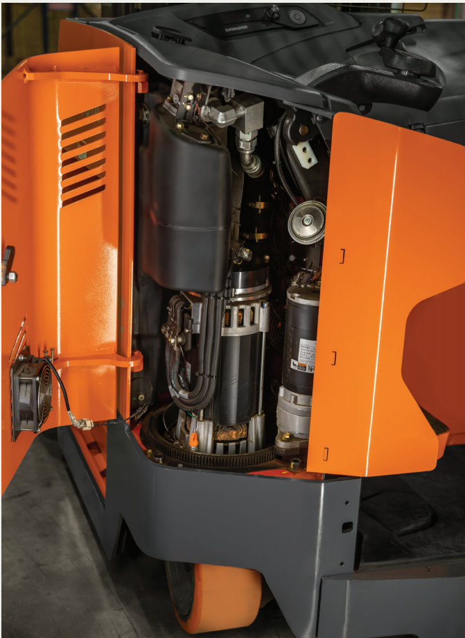
AC Drive and Lift Motor
